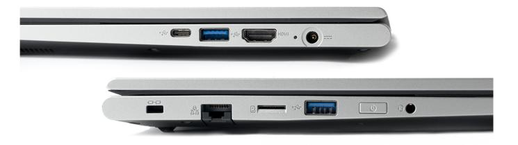
**1Gb LAN port:** When a little more speed is needed, and perfect for bulk imaging and deployment.
